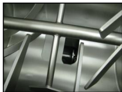
Grinder Opening Seals to Prevent Ingredients and Water from Falling into the Auger
