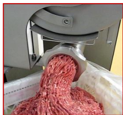
Grinder Opening Seals to Prevent Ingredients and Water from Falling into the Auger
