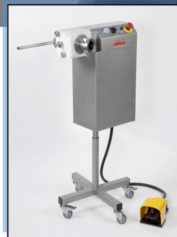
The PR-250 Mobile Stand makes connection to the Mainca "EM" stuffer fast and convenient. And the standard "EM" Knee Lever Lock allows for fully automatic operation of the PR-250
